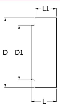
D = 480 D1 = 240 L = 190 L1 = 90 Max bore = 145 Torque (N m) = 16600
